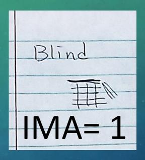
Advantage of the fixed pulley in blinds are that you do not need to pull each pieces together because it is controlled by pulley, even though it is only changing the direction of force (because the IMA is 1), it is making your life easier by making the movement done in one time.
