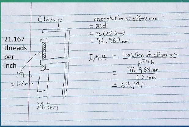
Clamp will make life easier by clamping things together with strong power using the screw. Clamp is using the screw because screw can make strong enough power to clamp things together and make it stable.
