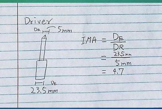
Drivers makes life easier by turning screws easier because it is almost impossible to turn screws by your own hand, and so this item is used because it will make 4.7 times less effort to turn the screws.
