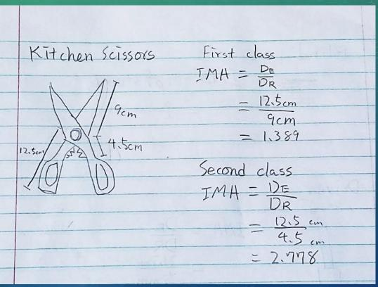
Kitchen Scissors will make life easier by cutting things with the First class levers (also increases powers by 1.389 times). And it will also make life easier by breaking or opening things with the second class levers, because the force applied to the objects will be increased by 2.778 times the force you will apply.
